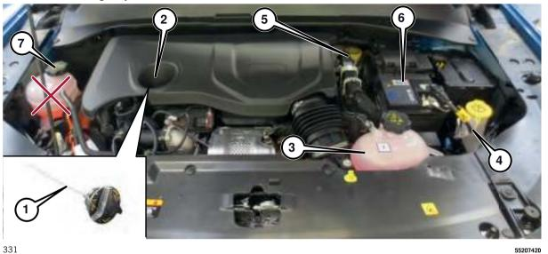
1. Engine oil level dipstick 2. Engine oil cap/filler 3. Heat engine coolant 4. Windscreen/rear window washer fluid 5. Brake fluid 6. Conventional battery 7. High-voltage system coolant
