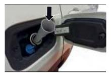
3. Ensure funnel is inserted fully to hold flapper door open.
