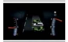
55208100 When the driver places the gear lever to the D (Drive) position (for automatic transmission) or in first gear (for manual transmission), the system may instruct the driver to wait for steering to complete.
