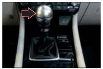
To engage the gears, press the clutch pedal fully and put the gear select in the required position (the gear engagement diagram is shown on the selector knob). To engage position R (Reverse) from position N (Neutral), lift the position ring, located under the knob and then move the gear selector all left and then forwards.
