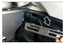
5. Push on the outer edge fig. 269 to open the fuel filler flap.
