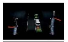
Your car is now in the parallel park position. The message notifying you of the completion of the parking manoeuvre is momentarily shown. When the manoeuvre is complete, the driver will be instructed to check the parking position of the car. When you is satisfied with the manoeuvre, set the automatic transmission in position P (Park) or the
