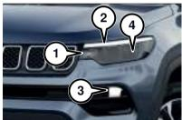
1. Front direction indicators (light bulbs or LED) 2. LED daytime running lights (DRL) and side lights 3. LED fog lights 4. Dipped beam / main beam headlights (LED)
