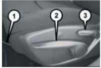
While sitting in the seat, pull up on the handle (1) fig. 21 and slide the seat forward or backward. Release the bar once you have reached the desired position. Using body pressure, push the seat back and forth to make sure the adjustment devices have locked.
