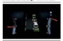
When the car has reached the end of its forward movement, the system will instruct the driver to check their surroundings and stop the car's movement.
