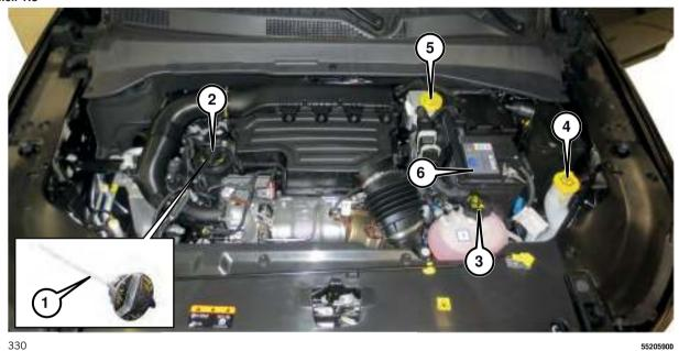
1. Engine oil level dipstick 2. Engine oil cap/filler 3. Engine coolant 4. Windscreen/rear window washer fluid 5. Brake fluid 6. Conventional battery
