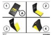
■ Then position the wedge (1) fig. 308 (where provided) or a stone at the rear. on the wheel diagonally opposite the wheel to be replaced so as to prevent unwanted movement of the car when it is raised off the ground;
