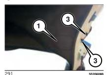
3. Undo the screws (3) fig. 291 and fig. 292 and remove the light cluster.
