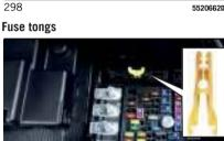
To replace a fuse, use the pincer fig. 299 under the engine compartment fusebox cover.
