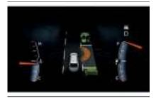
5520798D When an available parking space has been found, and the car is not in position, you will be instructed to move forward to position the car for a parallel parking sequence.
