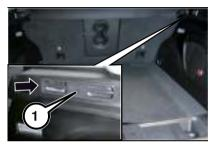
4. Grab the release cable tether fig. 276 and gently pull up to unlock the fuel filler flap.
