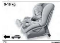
Children weighing between 9 and 18 kg can be placed on Group 1 child restraint systems facing the direction of travel, as shown in fig. 139. This type of restraint system is for older children who are too big for a Group 0 or 0+ child restraint system.
