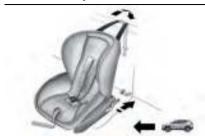
143 Your car is equipped with the child restraint anchoring system called ISOFIX. This system allows ISOFIX equipped child restraint systems to be installed without using the seat belts of the car. The ISOFIX system has two lower anchoring located at the back of the seat cushion where it meets the backrest and a top anchoring located behind the seat.
