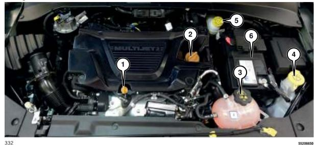
1. Engine oil level dipstick 2. Engine oil cap/filler 3. Engine coolant 4. Windscreen/rear window washer fluid 5. Brake fluid 6. Conventional battery
