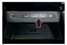
The car will start in "Electric" mode if this mode was selected the last time the engine was switched off, and if the conditions are right to enable it, including:
