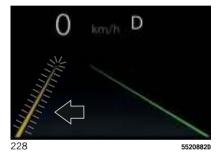
On versions with 10" display, LaneSense system notifications are kept visible in the lower right corner of the display even on screens other than the main LaneSense system screen fig. 229.
