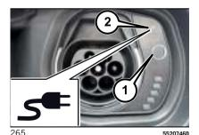
If, approximately 60 seconds after the doors are unlocked, the system detects that the charging cable is still connected inside the charging port, charging will restart automatically and the cable will be locked inside the charging port. A dedicated message will appear on the Uconnect™ system display.
