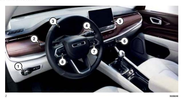
1. Headlight switch 2. Multi-function control stalk (headlights) 3. Instrument panel 4. Windscreen wiper stalk 5. Buttons (Emergency lights, ParkSense system, Active ParkSense system, LaneSense system, ESC system, eCoasting mode) and **Uconnect™**system 6. Climate control system 7. Driving assistance systems (Cruise Control, Adaptive Cruise Control, Speed Limiter, Intelligent Speed Assist) 8. Display control buttons, accept/reject incoming call, voice commands
