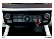
These USB ports have a "Smart Charge" feature that allows you to charge your connected device for one hour until the engine is turned off.
