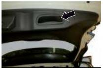
NOTE Use the door lock button from the inside or on the key to close the liftgate. Closing the doors using the outer latch does not lock the liftgate.
