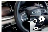
To carry out the adjustment move the lever (1) fig. 29 downwards in position (A), then adjust the steering wheel to the most suitable position and then lock it in this position moving the lever (1) again in position (B) to lock it entirely
